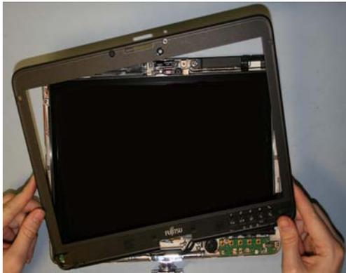
45. Use a plastic Pry Tool to remove the LCD front cover.
