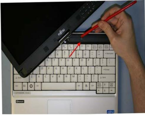
17. Remove screw covers from right and left sides of LCD.
