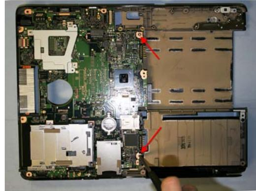
36. Remove 2 screws securing System board.
