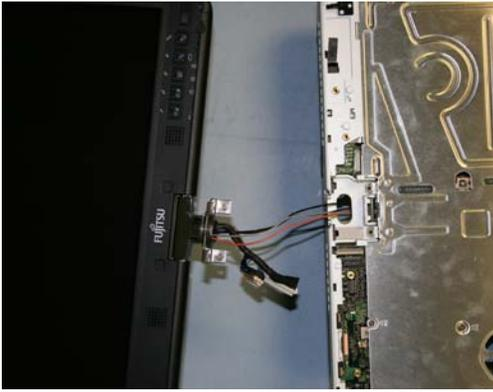
29. Remove LCD assembly from Lower assembly.
