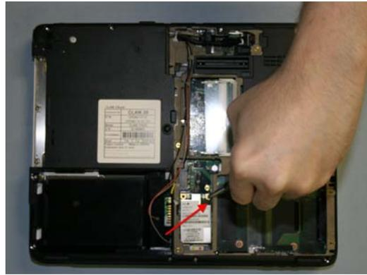
14. Remove 1 screw securing WWAN card and remove card.
