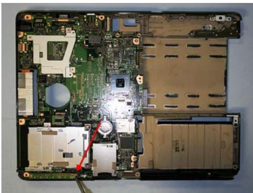
32. Replace LED board and secure with 1 screw.
