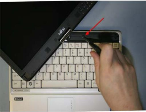
48. Replace Hinge cover and secure screws on the right and left sides of the LCD.
