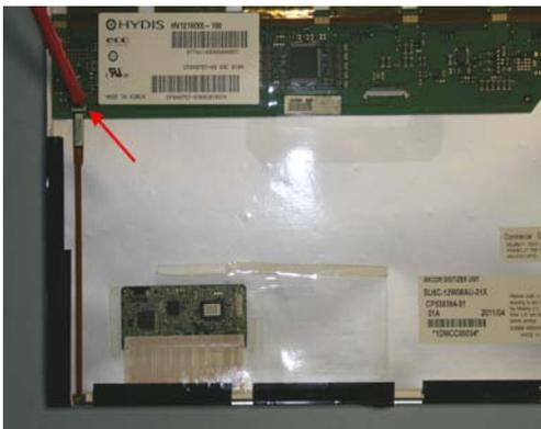
53. Disconnect Flex cable from LCD control board.
