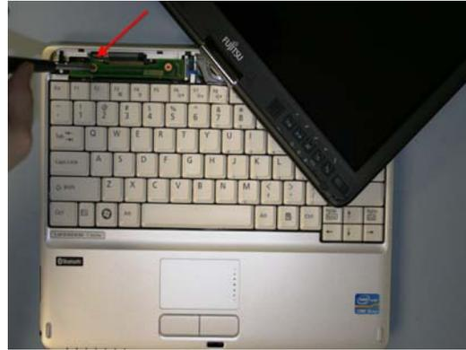
20. Remove 1 screw securing Rotation board.
