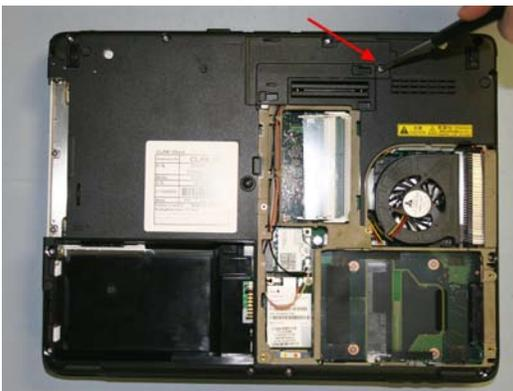
56. Replace LCD cable cover and secure with 1 screw.
