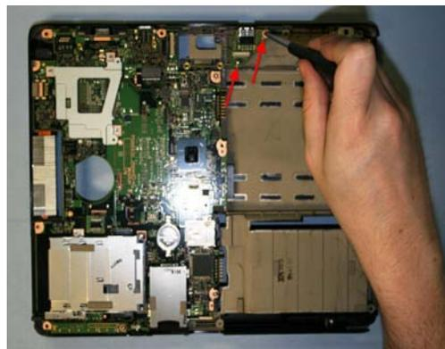
33. Replace USB board and secure with 2 screws.
