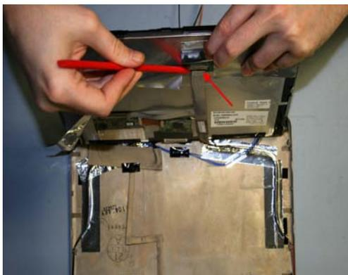
47. Remove tape securing LCD cable and disconnect LCD cable.
