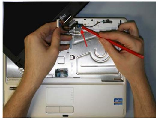
24. Disconnect USB cable from System board and USB board and remove cable.
