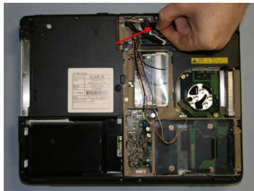
28. Disconnect LCD cables from the System board.
