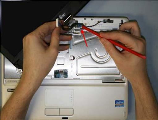
42. Connect USB cable to System board and USB board.
