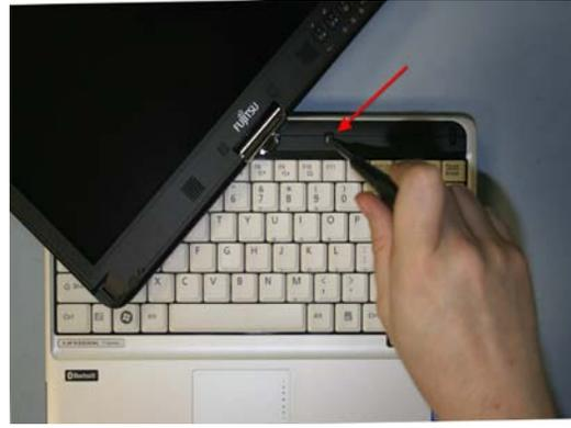
18. Remove screws from right and left sides of LCD and remove front Hinge cover.
