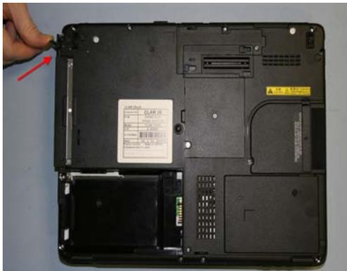
3. Eject and remove the Optical Drive.
