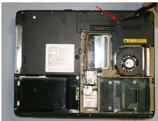
10. Remove 1 screw from the LCD cable cover and remove cover.
