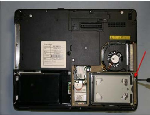
60. Replace Hard Drive and secure the Hard Drive with 1 screw.
