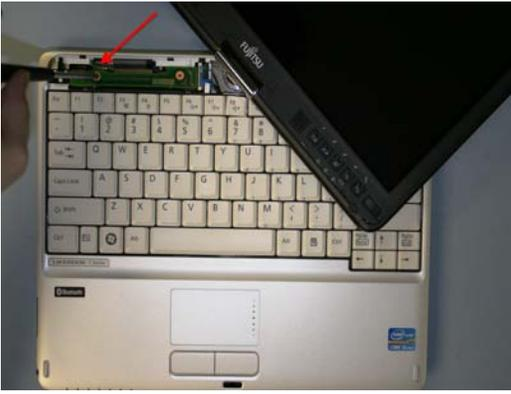
46. Replace Rotation board and secure with 1 screw.
