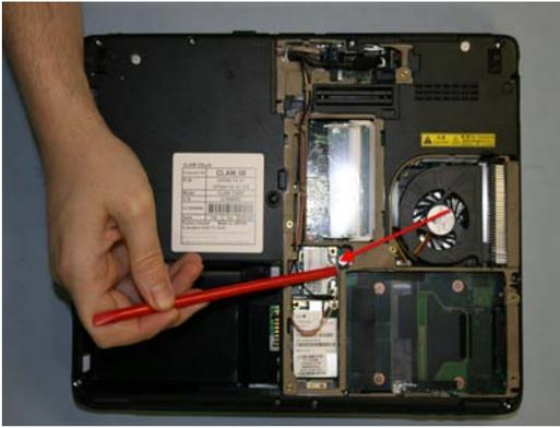
11. Disconnect cables from WLAN card.
