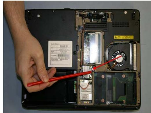
55. Connect cables to the WLAN card.
