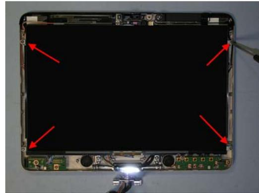
46. Remove 4 screws securing LCD.
