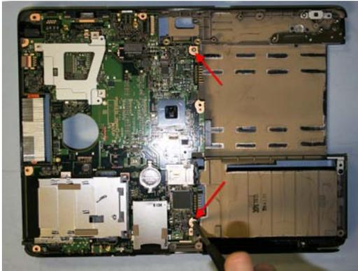
30. Replace 2 screws to secure the System board.
