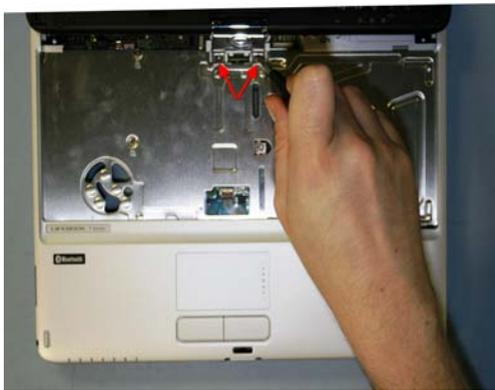
25. Remove 2 screws securing Hinge.
