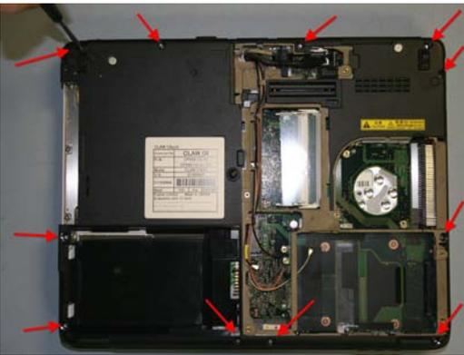
50. Replace 11 screws securing the Lower assembly.
