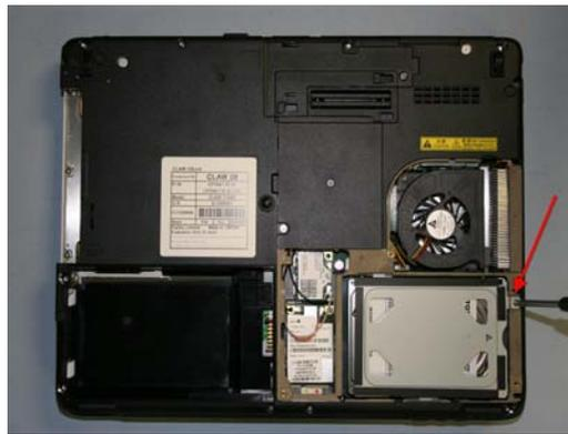
6. Remove 1 screw securing Hard Drive and remove the Hard Drive.
