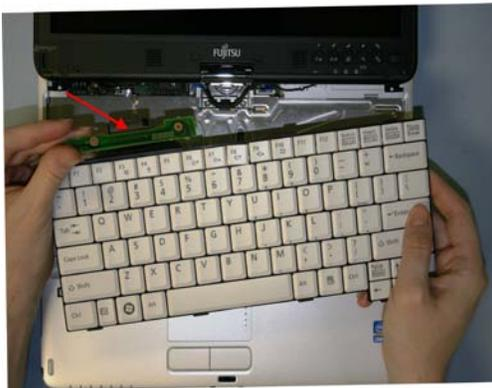
21. Remove Rotation board and Keyboard from System board.
