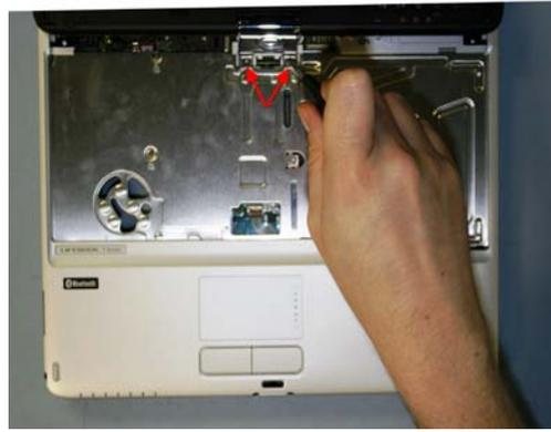
41. Replace Hinge and secure with 2 screws.
