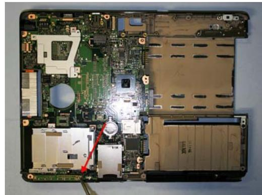
34. Remove 1 screw securing LED board and remove board.
