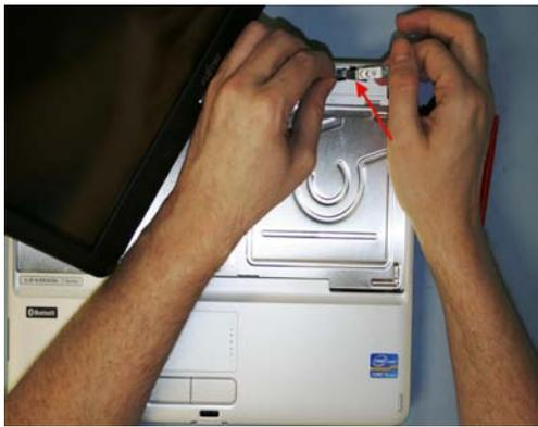
23. Lift up Bluetooth board and disconnect cable.
