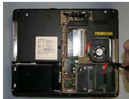
15. Remove 2 screws securing Fan and remove Fan.
