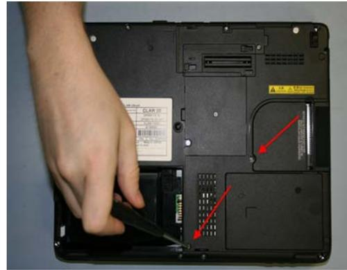
61. Replace Hard Drive cover and secure with 1 screw.
