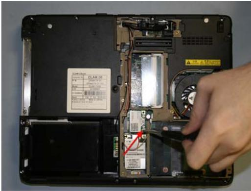
54. Replace WLAN card and secure with 1 screw.
