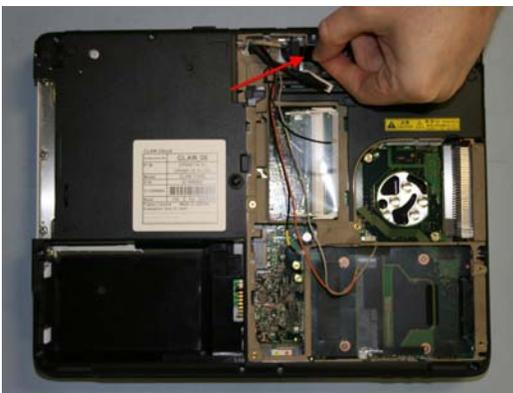
38. Connect LCD cables to the System board.
