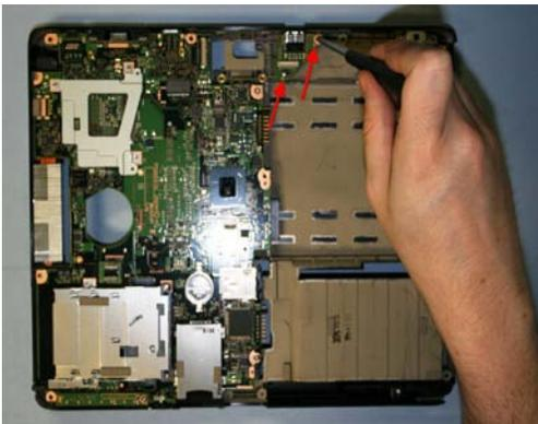
33. Remove 2 screws securing USB board and remove board.
