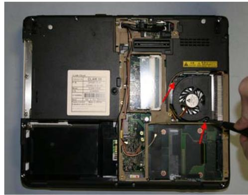
51. Replace Fan and secure with 2 screws.
